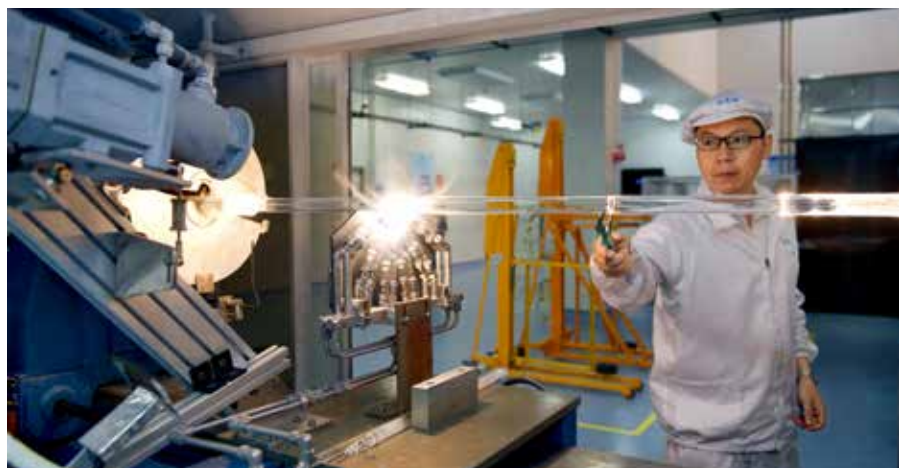
A worker from Fasten Group makes optical fiber robs at the Modified Chemical Vapor Deposition facilities. by Chen Ye
